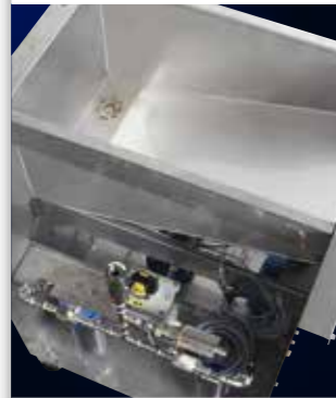
60 L Tank with filter and piping
