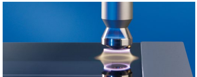
Openair-Plasma® pretreatment: oven glass before handles are bonded
