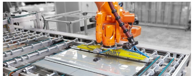
Adhesive bonding of the components to the treated surface © Benteler GmbH
