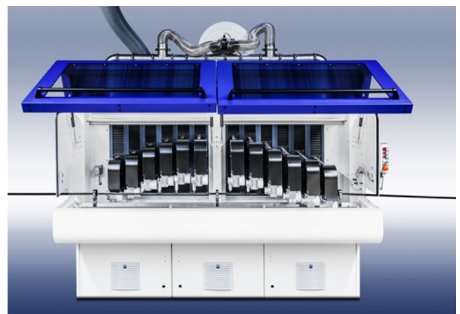
Fully automated plasma system - "Plasmatreat Exact" with 12 jets
