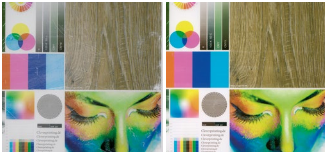
Left: Printing on glass without Openair-Plasma® treatment. Right: With Openair-Plasma® the printing quality is substantially improved.
