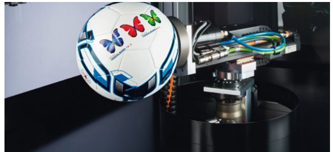
By using the Openair-Plasma® technology, long-term printing results are possible, even on objects that are exposed to high mechanical loads. Picture: Heidelberg Druckmaschinen AG
