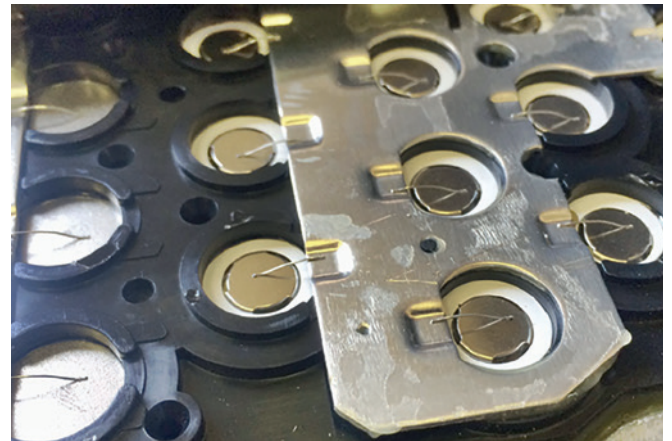
Bonding pad: Microfine cleaning of the contact surfaces with Openair-Plasma®.
