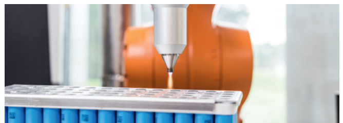
Openair-Plasma® treatment of cylindrical and pouch cells
