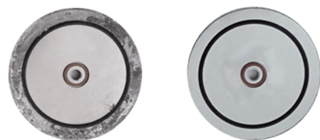
Comparison after 960 hours salt spray test: AlSi12 alloy without (left) and with PlasmaPlus® coating (right)
