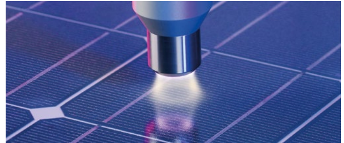
Openair-Plasma® treatment of the glass surface
