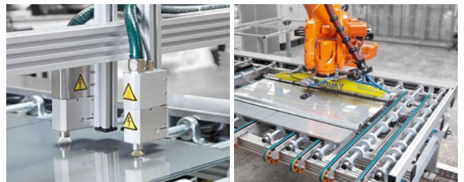
Fig. left: Openair-Plasma® pretreatment of the panel Fig. right: Adhesive bonding of the components to the treated surface Source: Benteler Maschinenbau GmbH
