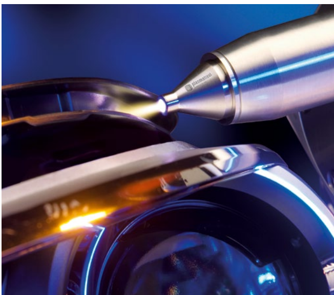
Gap-filling plasma treatment of headlight housing
