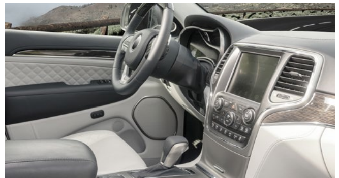
Use of multi-component soft touch parts in the automotive industry: Dashboard, interior door panels and gear knob. © Covestro AG / Media-Assistent
