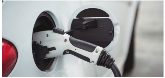
Hard-soft composites satisfy diverse electromobility requirements: In charging plugs, thermoplastics provide mechanical strength while elastomers provide good grip and high media resistance.
