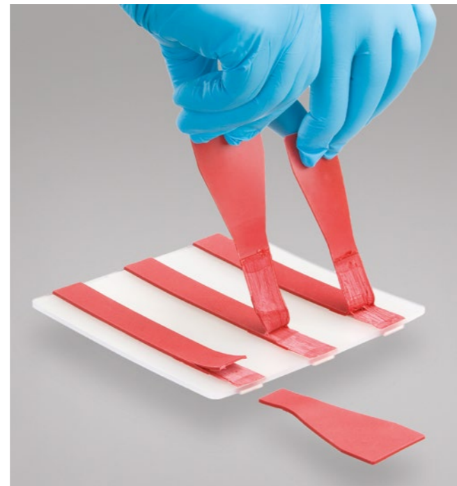
2-component peel test specimen made from TPU and PP – complete cohesive failure of the elastomer component (TPU – Desmopan 6064A on PP – Purell HP 570M), both not adhesion modified
