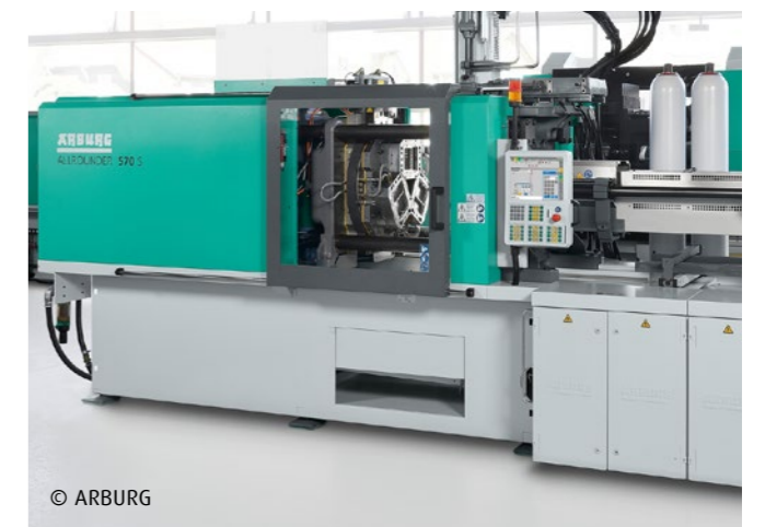
InMould-Plasma® mold integrated into an ARBURG Allrounder 570S.
